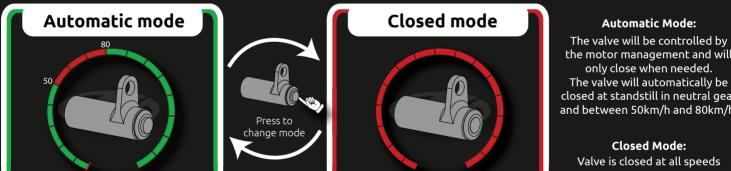
the motor management and will only close when needed. The valve will automatically be closed at standstill in neutral gear and between 50km/h and 80km/h.
